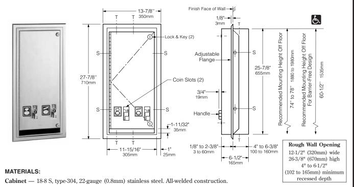
**Flange** — 18-8 S, type-304, 22-gauge (0.8mm) stainless steel with satin finish. Drawn and beveled, one-piece, seamless construction. Adjustable escutcheon-type flange permits semi- or fully-recessed installation.
