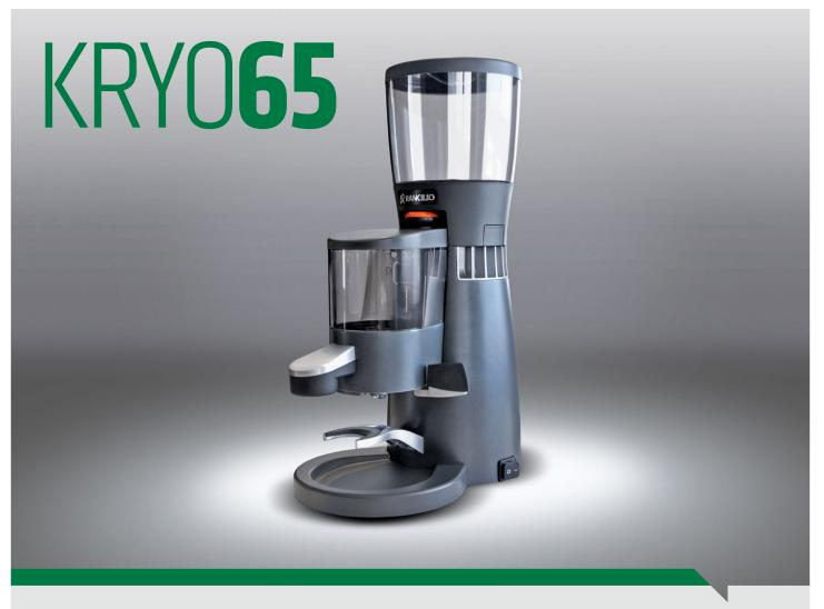
**KRY065** is fitted with 2.5 inch (64mm) diameter mills, ensuring a production of 15-20 lb/h (7-9 kg/h). The dose can be regulated between 0.19 and 0.35 oz (5.5-10 g), with a coffee bean capacity of 2.9 lb (1.3 kg). It is available in an automatic (AT) or semiautomatic (ST) version.
