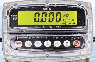
The Admiral's keypad senses the operator's finger from inside the enclosure, thus eliminating the need for any opening in the front of the IP69K-rated indicator. A red status LED for each key signals to the operator that their touch has been received. There are no moving parts to wear out or exposed electronics in the scale's indicator.
