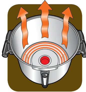
Dual Heater System Center Heater brews coffee, then shuts off. Gentle Warming Heater keeps coffee at a constant serving temperature without overcooking it.
