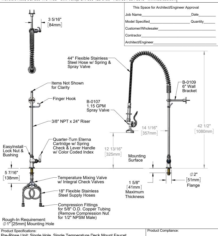
Pre-Rinse Unit: Single Hole, Single Temperature Deck Mount Faucet, Quarter-Turn Eterna Cartridge w/ Spring Check, Lever Handle, 24" Riser, Wall Bracket, 44" Flexible Stainless Steel Hose, 1.15 GPM Spray Valve, Temperature Control Mixing Valve w/ Integral Check Valves & 18" Flexible Stainless Steel Supply Hoses w/ 1/2" NPSM Male Inlets
