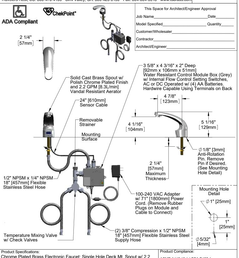
Chrome Plated Brass Electronic Faucet: Single Hole Deck Mt. Spout w/ 2.2 GPM VR Aerator, AC/DC Control Module w/ Internal Flow Cont. Setting Switches, Temperature Cont. Mixing Valve w/ Check Valves, 18" Hot & Cold Supply Stop Flexible Connector Hoses
