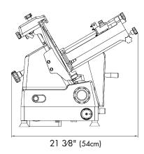
Controls: Manual slice thickness knob, push button on/off, attached blade sharpener, smooth cam auto/ manual knob
