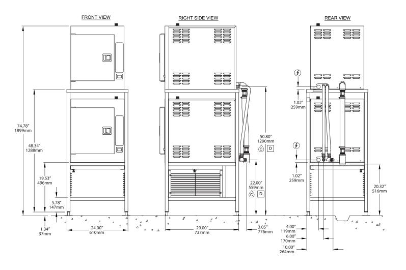
\*NOTES: The diagrams above are shown with the model 21-CET-8 mounted on the ES-2446 Stacking Equipment Stand.
