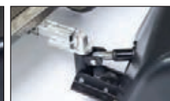
Hitches dock easily to coupling on the tug
