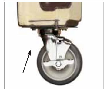
CASTER IMPACT PLATES Impact plates add metal reinforcement to hold casters in place even when dropped.
