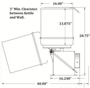
6" Recommended Min. Clearance between wall and Cntl Box for Service.
