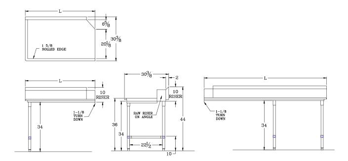
All units ship unassembled for reduced shipping cost. Units 7 ft. and larger are furnished with four legs. All dimensions are typical.
