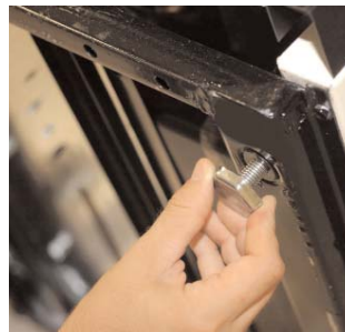
Leg levelers are height adjustable by tightening or loosen the leg lever.
