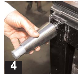
4 Thread leg into cabinet bottom frame rail.
