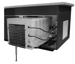
Slide-out accessory for Satellite-fill Maestro icemakers facilitates installation and service. Utility distribution panel allows easy connection of electric, incoming water and drain. Flexible connections from panel to icemaker allow icemaker to slide out for cleaning and service without disconnecting utilities. Includes front leg to support icemaker.
