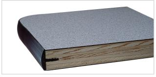
Solid 3/4" thick plywood is surfaced with high pressure plastic laminate, sealed with a backing sheet and edged with vinyl T-molding.
