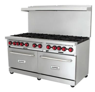
This commercial gas range has powerful Planck 30,000 BTU cast iron burners. Each burner has a lift off head - individual pilot light - heavy duty 12" x 12" removable cast iron grate and individual instant light control knob. It is constructed with a stainless steel front, 24.75" high backriser and shelf, 6" adjustable stainless steel legs or casters and a  $\frac{3}{4}$ " NPT gas connection.
